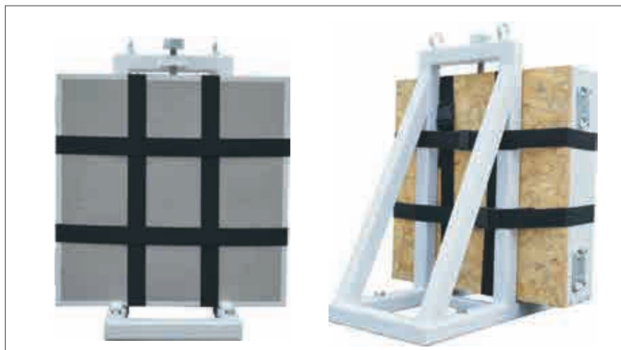
Assembly of Backing Material Fixture and Backing Material Holder
